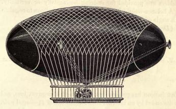
or blower, which is actuated by the aëronaut or by a suitable motor.
